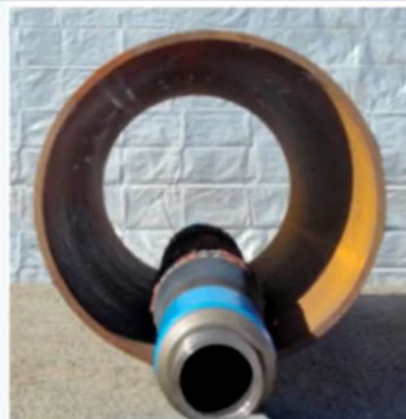
STAINLESS PATCH SWAGED 360° AGAINST THE CASING
